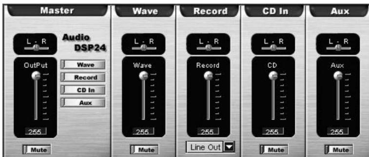
You can control the systems internal components with the *Internal Mixer*. The *Internal Mixer* works basically like a normal soundcard and can be used for standard multimedia software or games for example. Please see the following section with more details:
