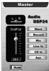
You can control the panning and the master volume. Muting the signal is possible as well.
