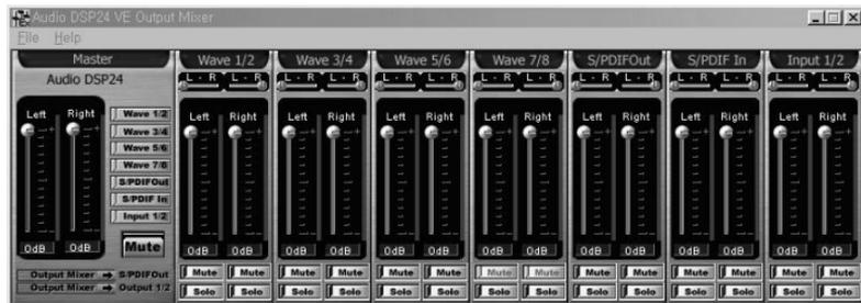
**Note:** The *Output Mixer* will only change the audible signal. You can output it either through Output 1,2 and/or through the S/PDIF Output (setup under *Master*). When you are recording an input signal, the *Output Mixer* does not change the signal level. This ensures that you are always recording with best possible quality.
