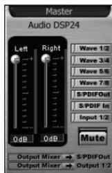
You can control the the volume of the left and right channels independantly. Muting the signal is possible as well.
