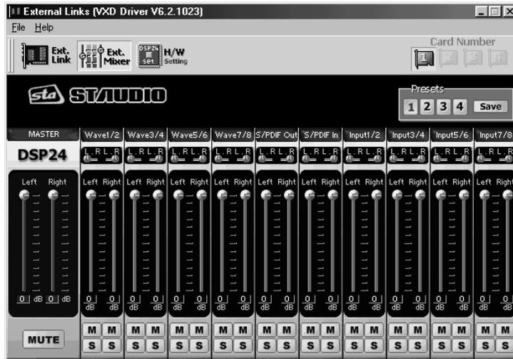
**Note:** The *External Mixer* will only change the audible signal for monitoring purposes. You can either output it through the analog output 1/2 and/or through the S/PDIF output (as connected inside *External Links*). When you are recording an input signal, the digital *External Mixer* does not change the signal level. This ensures that you are always recording with best possible audio quality without reduction of the dynamic range.
