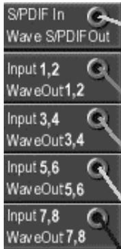
The five gray virtual connectors in the middle section are corresponding to the MME wave devices (and the ASIO-driver) you are using inside your application.
