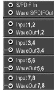
All of these available signal sources can be connected to the outputs on the left side of the *External Links* window.
